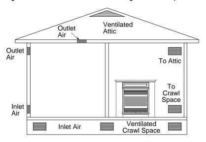
Figure 6 - Ventilation Air from Outdoors Shown with Optional Mantel
